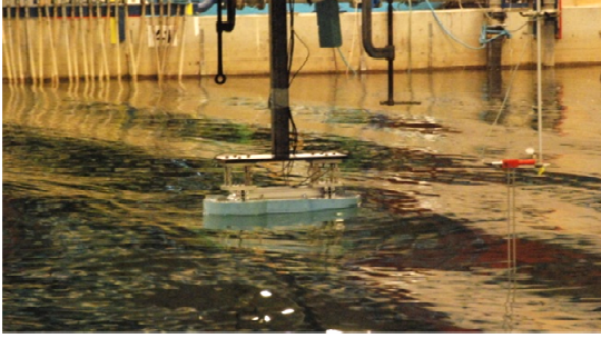
Fig. 4 The first experimental setup is concerned with the wave excitation forces. The buoy is rigidly fixed at draft d (see Table I). Two force transducers are mounted between the buoy and a rigid beam, and the wave elevation is measured in parallel with the buoy (the wave measuring device can be seen to the right in the figure).
